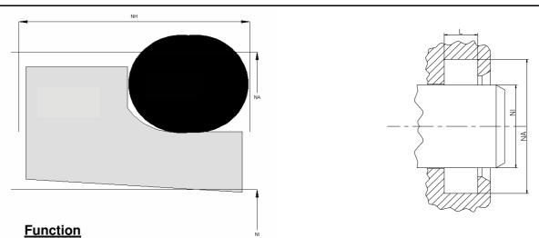
Wipers are designed to keep dust, dirt, sand and others off the rod and the sealing and guiding elements, avoiding abrasive damage caused by external contamination.
