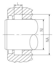
Rod seals are designed to seal the pressurized hydraulic fluid against the atmosphere, preventing leakage and pollution of the environment.
