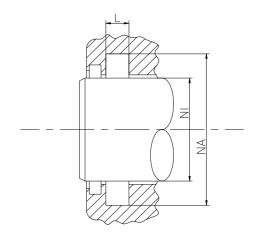
Rod seals are designed to seal the pressurized hydraulic fluid against the atmosphere, preventing leakage and pollution of the environment.
