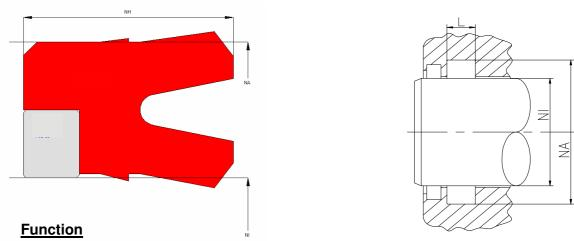
Rod seals are designed to seal the pressurized hydraulic fluid against the atmosphere, preventing leakage and pollution of the environment.
